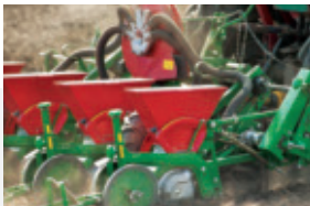
Independent control of each seed drop, made possible by Elliott's flexible shaft technology, eliminates waste saving farmers money.
